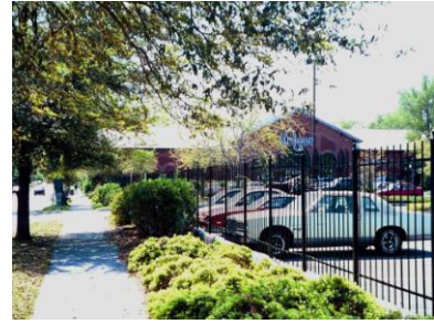
Screen parking lots from the street with a brick wall, wrought-iron fencing, and/or landscaping
