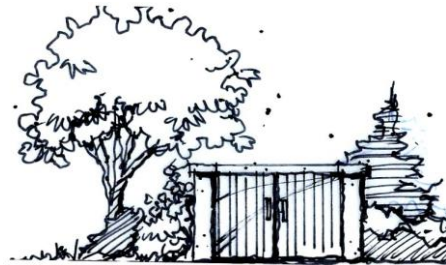
Image depicting appropriate screening requirements of dumpsters.
