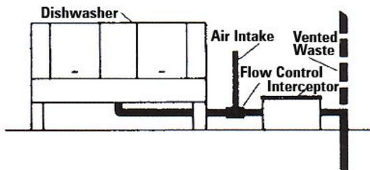
Figure A1.5.3- Interceptor Serving Dishwasher-Flow Control Air Intake Terminates Above Flood Level
