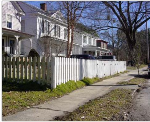
Figure 33: Simple, narrow sidewalks with a small grass strip separating them from the street would improve pedestrian safety in Jersey City.
