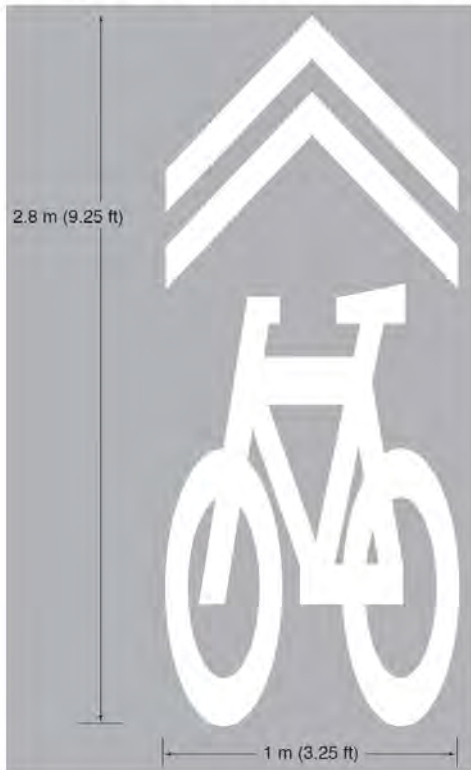
Figure 9C-9. Shared Lane Marking
